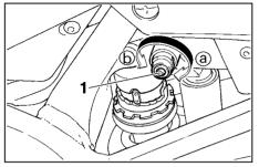
1. Compression damping force adjusting screw
